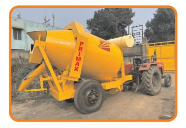
A transit mixer is a multipurpose device that is used to transport concrete mortar from a concrete batching plant. The transit mixer consists of a drum with a spiral blade that has the ability to move in two directions.
