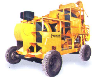
Mobile Hot Mix Plant
