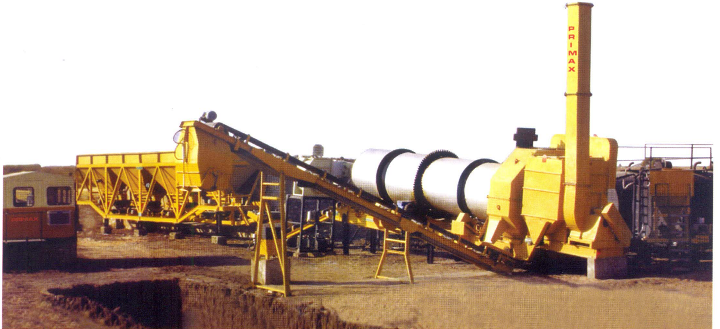
ASPHALT DRUM MIX PLANT
